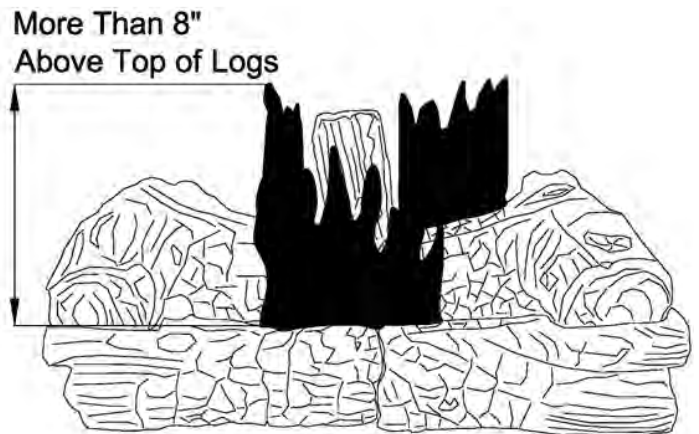
Fig. 25—Incorrect Burner Flame Pattern
